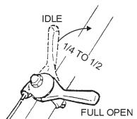
Figure 6. Throttle Lever (1/4 to 1/2)
